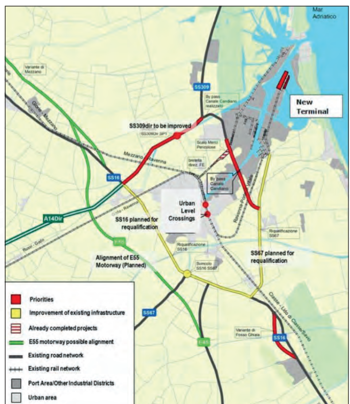
Figure 5 - Port last mile connections
