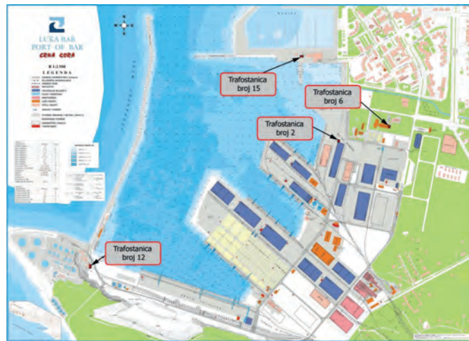
Figure 40 - Position of the substations
